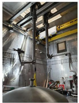
Manipulator for maintenance work at the fuel handling cell
